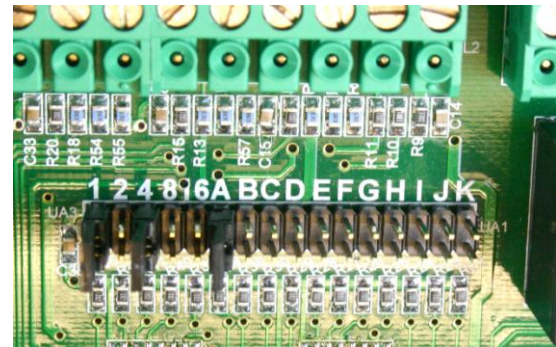
Jumpers A, 1 and 4 are ON (stand-alone mode, with damper group 1 to 5 in use)
